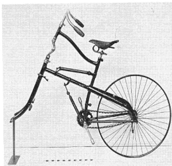
Figura 3: Whippet Spring Frame (1885) (15)
